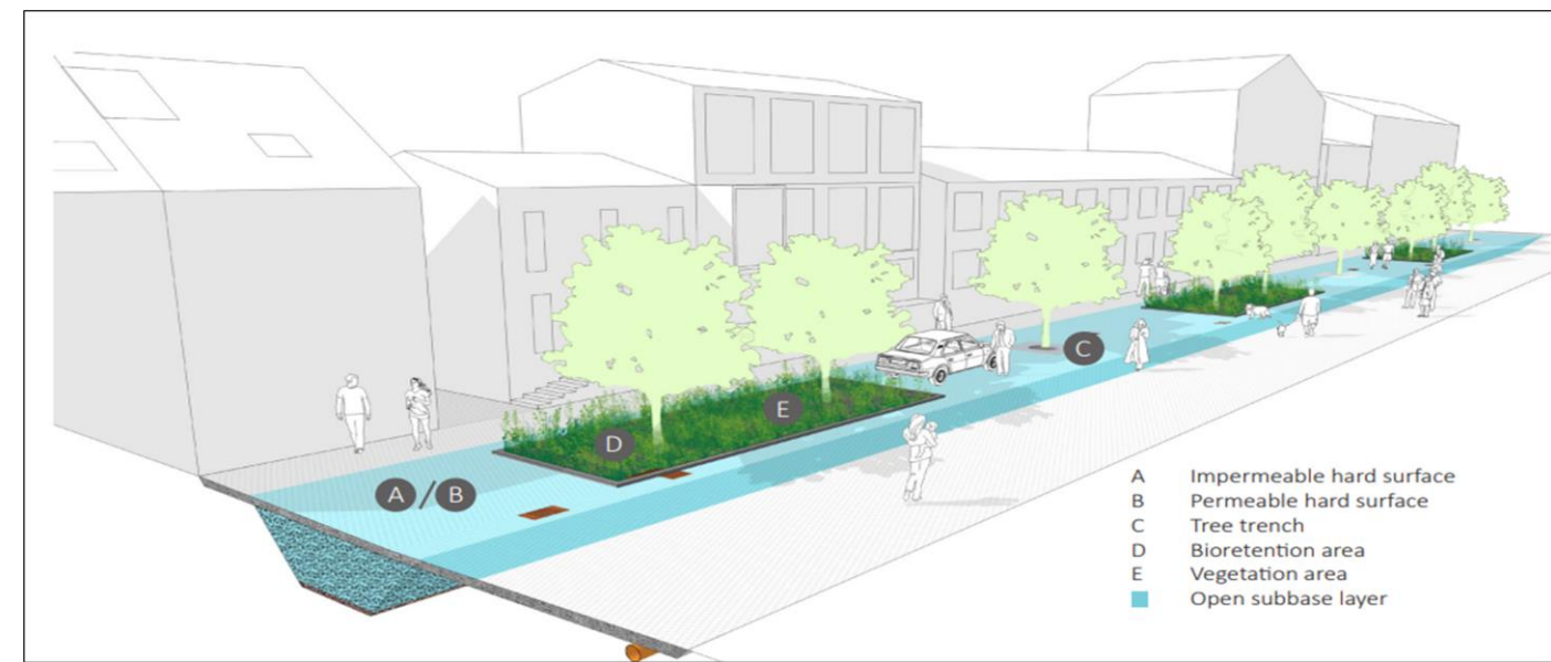
Figure 1 – Conceptual presentation of the proposed LID to mitigate pluvial flood risk for future challenging climate (source: Liveable-Streets-A-Handbook-of-Bluegreengrey-Systems, 2020)
